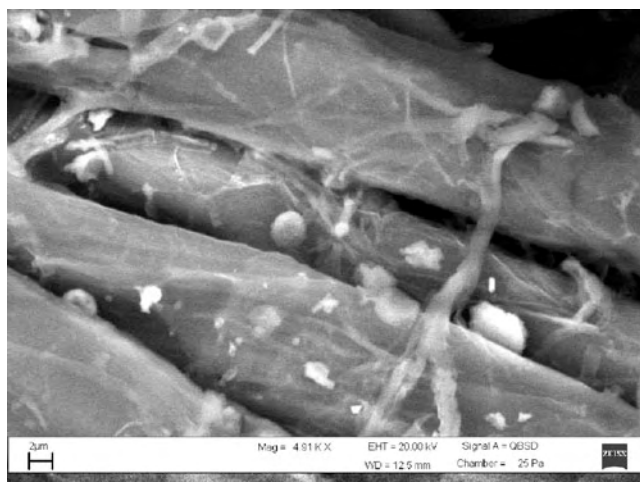
Figure 4 Scanning electron micrograph obtained with a backscattered electron detector (QBSD) in Variable Pressure mode
