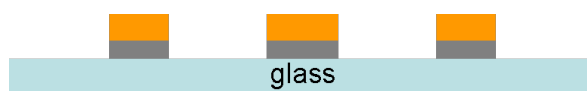
Figure 4.6: Illustration of the chrome etching process. Chemical etching removes unprotected chrome on the surface of the sample.
