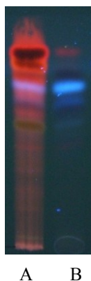
Figure 16 TLC: A: F1/2 with chlorophyll ; detection: under \text{UV}_{366} ; solvent system 4 B: F1/2 without chlorophyll ; detection: under \text{UV}_{366} ; solvent system 4
