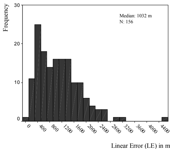
Figure C.1.2. Linear error (LE) between true locations and locations estimates by three bearings. The Andrews estimator was used for location estimation.
