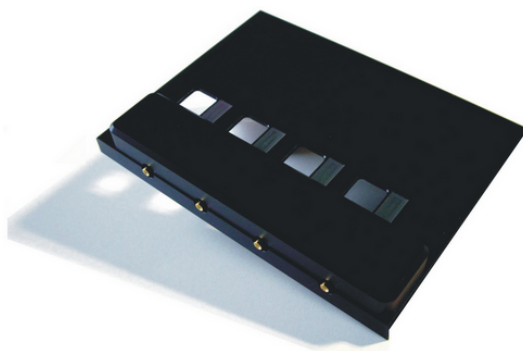
Figure 31: Platform with four integrated SAW-pumps for flow studies in microchannels.
