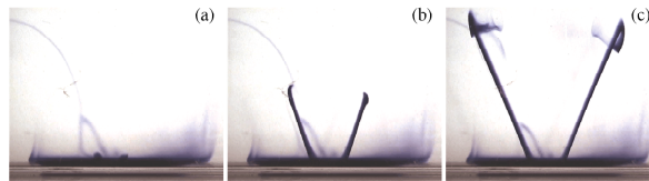
Figure 24: Dye at the interface between a piezoelectric substrate and a fluid is ejected by pressure jets of a surface acoustic wave (SAW). Image by courtesy of T. Franke, University of Augsburg
