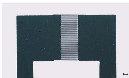
Figure 27: Interdigital transducers (IDTs). Bar represents 100 \mu\text{m} .
