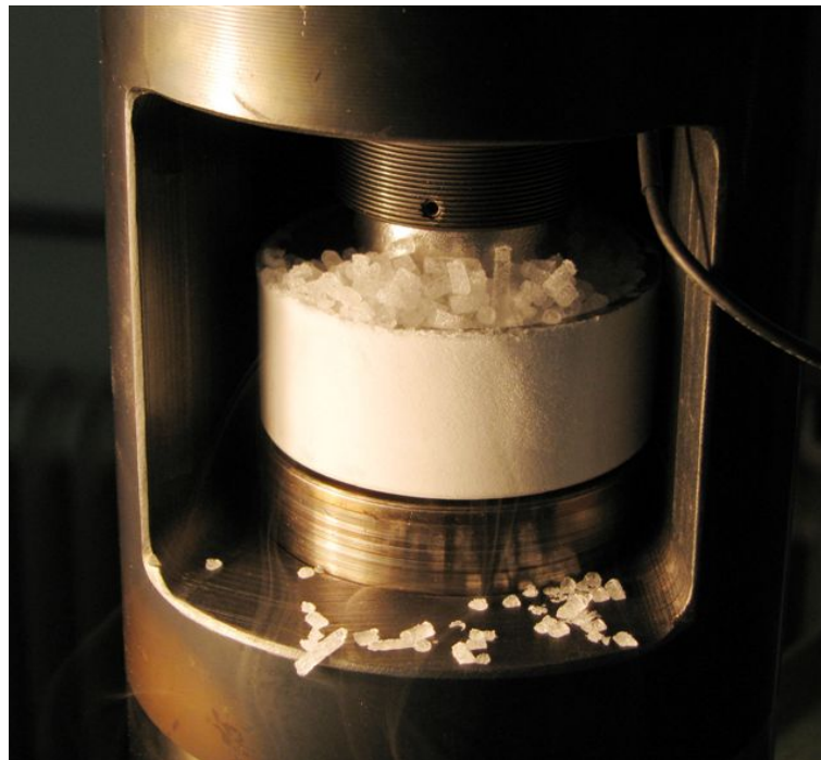
Figure 3.8: CO 2 cooling during HPT deformation.
