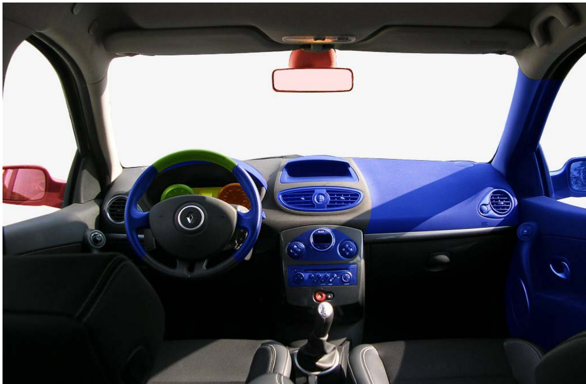
Figure 8.24 Map illustrating the relevance of the components of the Clio interior during driving tasks.
