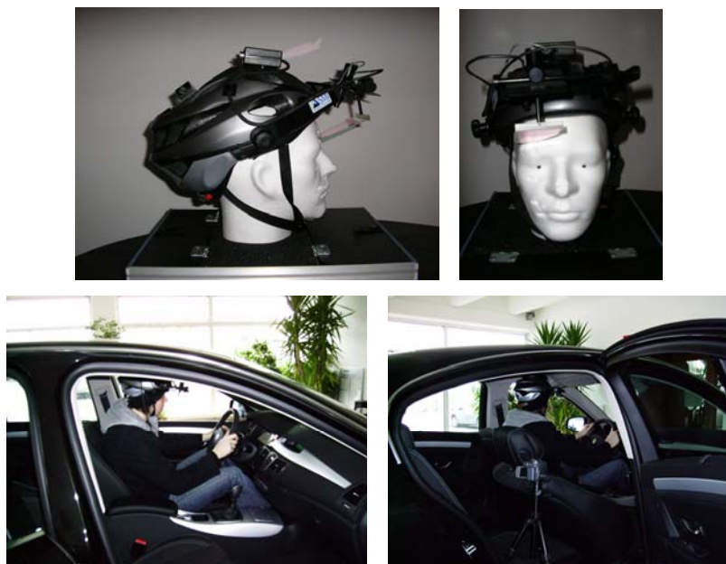
Figure 7.4: Images of the portable eyetracking device (upper row) and a subject wearing the device and sitting in one of the stimulus cars (lower row).
