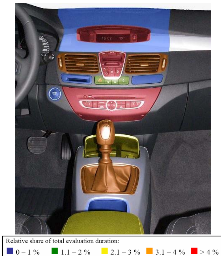
Figure 8.21 Map illustrating the relevance of the components of the centre-console and the gearshift area of the Laguna interior.
