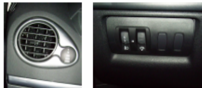
left ventilation shaft, control of headlights,
