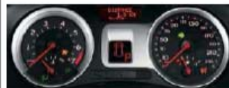
tachometer (left), dashboard display (middle), speed indicator (right), lining of instrument panel
