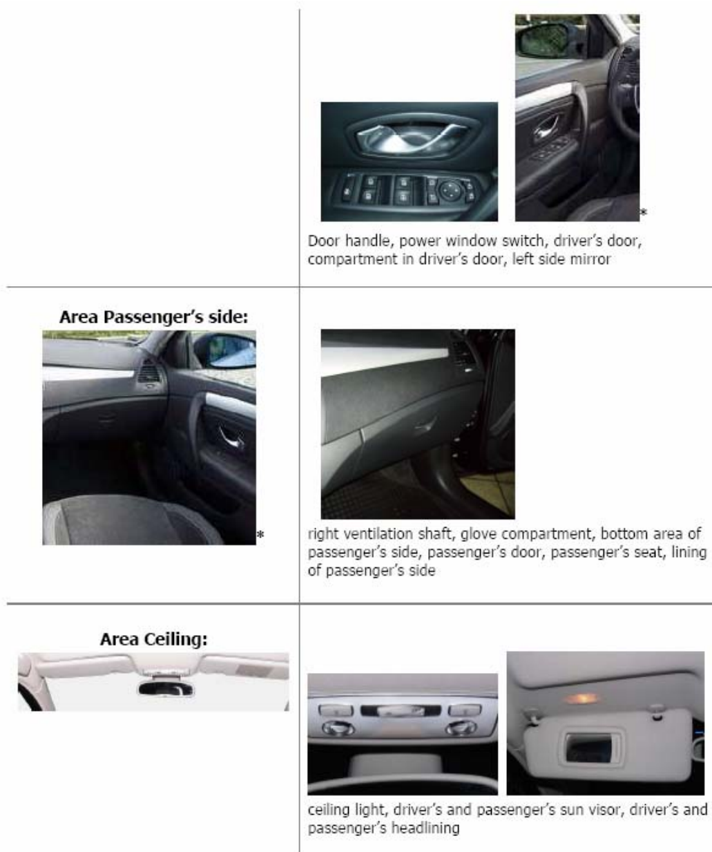
Figure 7.7 Images of the Laguna interior equipment and the components of the defined areas of interest.
