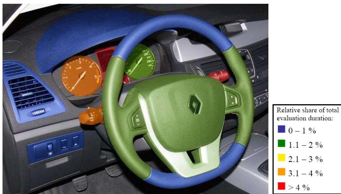
Figure 8.19 Map illustrating the relevance of the components of the instrument panel, the steering-wheel and parts of the left side of the Laguna interior.
