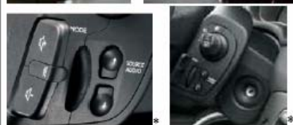
steering wheel, right and left multifunction switch (upper row), car radio control and key hole (lower row)
