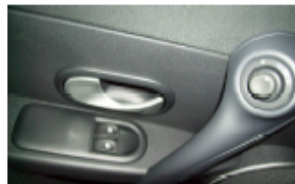
Power window switch. control of side mirror. door handle
