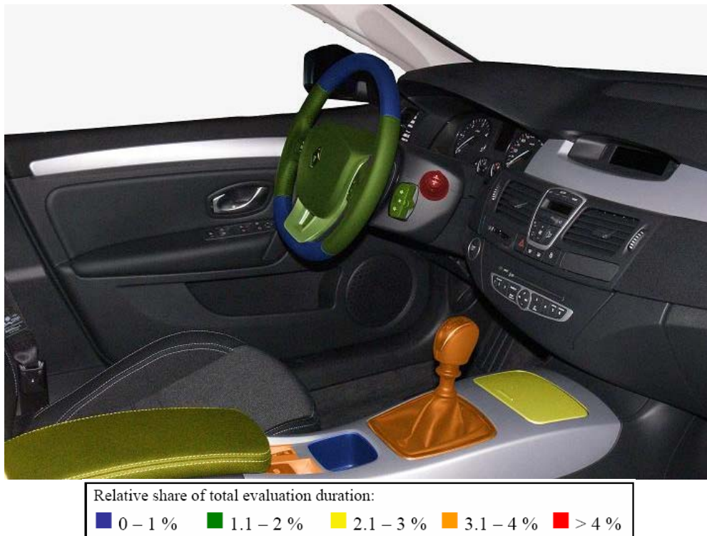
Figure 8.20 Map illustrating the relevance of the components of the gearshift area and the steering-wheel of the Laguna interior.
