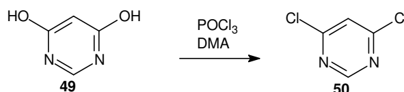
Scheme 13. Synthesis of 4,6-dichloropyrimidine 50
