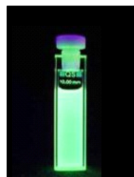
Figure 4: Fluorescence of azaphenothiazines at 364 nm
