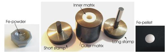
Figure 5.1: The left picture shows a natural iron powder in a mortar. The powder is then filled into the sample press and closed with the longer stamp in the middle picture. The right picture shows a typical iron pellet of 6 mm in diameter
