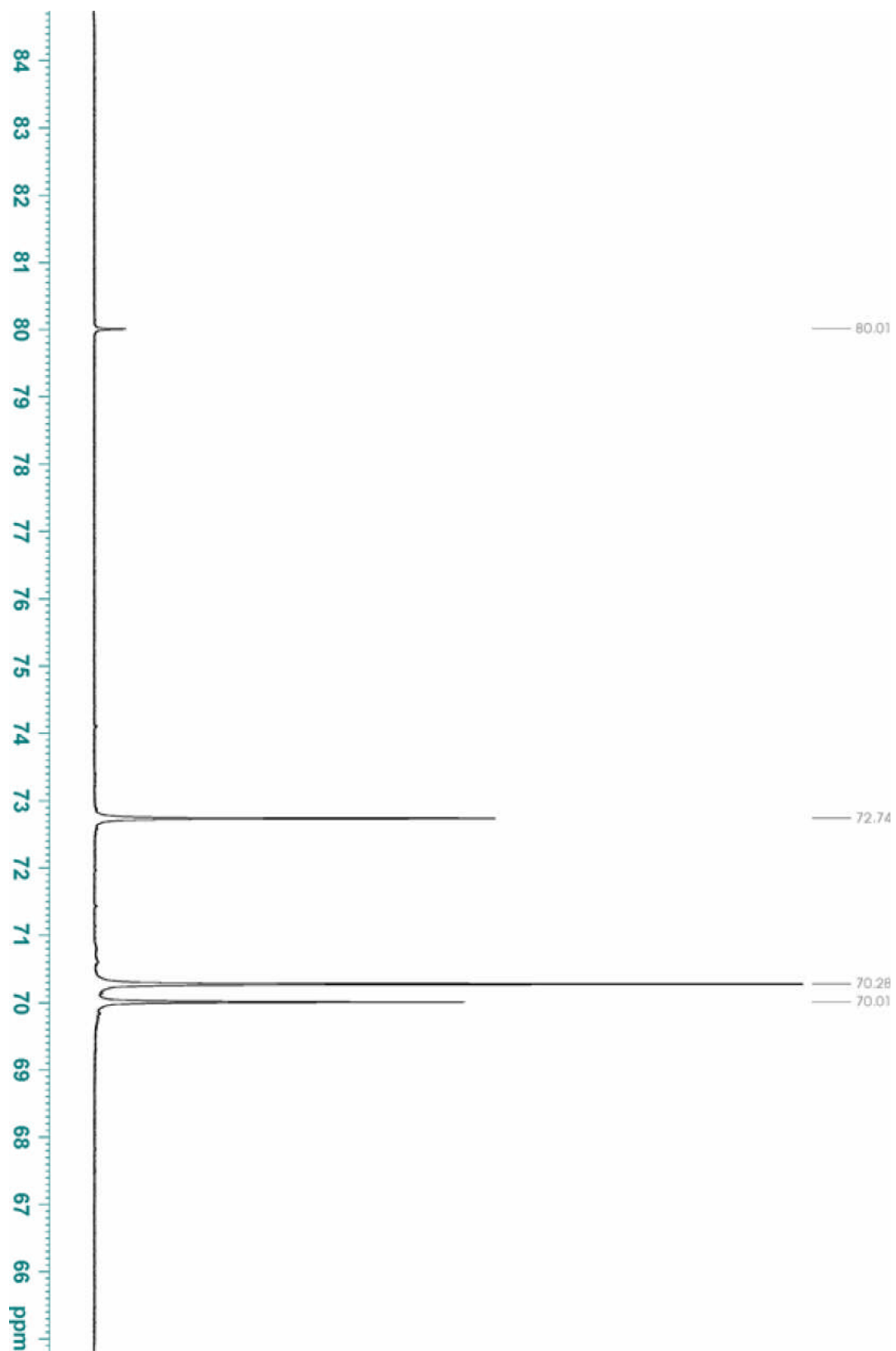
Figure S 4. 600 MHz ^{13}\text{C} NMR Spectrum of acetyl ferrocene in d_6 -DMSO at 300K.
