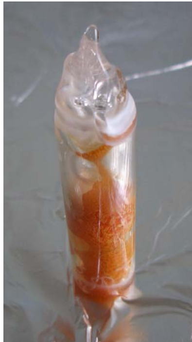
Fig. 3.1: Effect of P-evaporation during annealing: quenching resulted in the condensation of a huge amount of P on the inner quartz glass wall (Ni-P alloy containing 70 at.% P).
