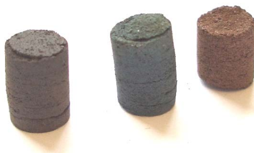
Fig. 4.7: Ni-P samples NP 33, 34 and 38 with 67, 69 and 74 at.% P (from left to right); these samples were prepared from powders of Ni and red P, pressed into pellets and annealed at 700 °C: their clearly non-metallic appearance is evident.
