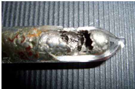
Fig. 3.2: Ni-P sample annealed at 900 °C. The sample is hollow due to evaporation of P.
