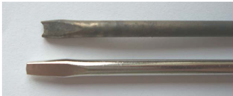
Fig. 1.2: Image of a solder tip of a commercial 20W soldering iron destroyed by use with Sn 3.8Ag 0.7Cu solder. A comparison with the length of a new tip shows the amount of material dissolved during soldering. There was no mechanical influence in the destruction of the tip.
