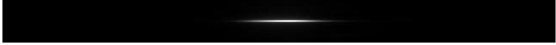
Figure A.3.: A spectrogram picture taken by the Deep Sky Imager CCD Camera. It shows the spectrum of a 4nm interference filter at 810nm. The number of illuminated pixels in the horizontal axis depends on the spectral width of the diffracted beam.
