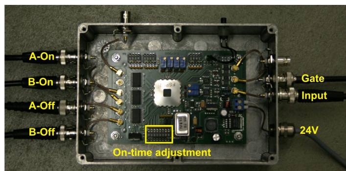
Figure 4.14.: A picture of a so called "splitter box" from the company Bergmann Meßgeräte KG. The input signal can be gated with another signal e.g. from a quantum random number generator (QRNG). The four output connectors on the left hand side transmit the control signals to the Pockels Cell. The On time of the Pockels Cell can be adjusted by several switches inside the "splitter box".
