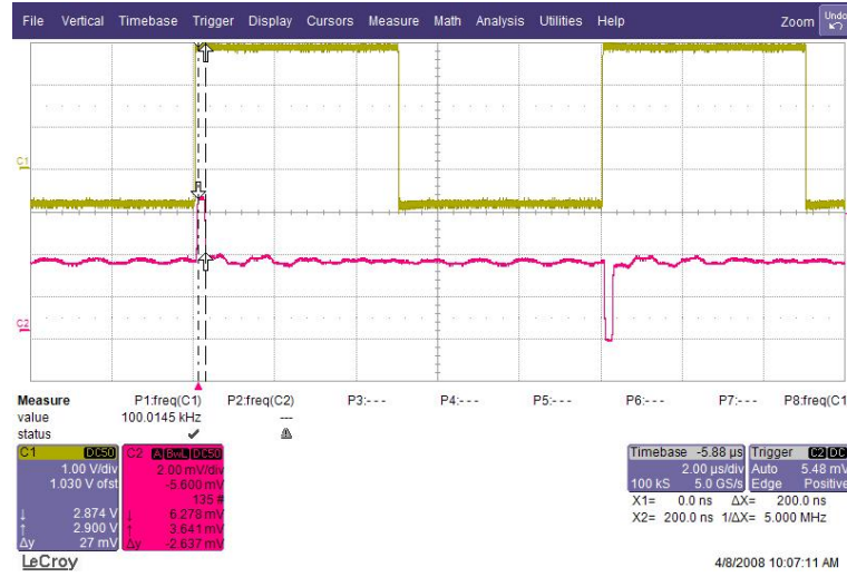
Figure 6.14.: A snapshot of the oscilloscope display, showing the optical switching behaviour of our Pockels Cells, which was placed in between two polarizers as described in the main text. The yellow curve shows the 100 kHz trigger signal, alternately applying positive and negative half wave voltage for 200 ns. This type of operation resulted in a high and low signal on the photodiode (red curve). In between a positive and a negative voltage pulse, no electric field was applied and half of the light intensity reached the photodiode. One can also see slight piezoelectric ringing after a voltage pulse.
