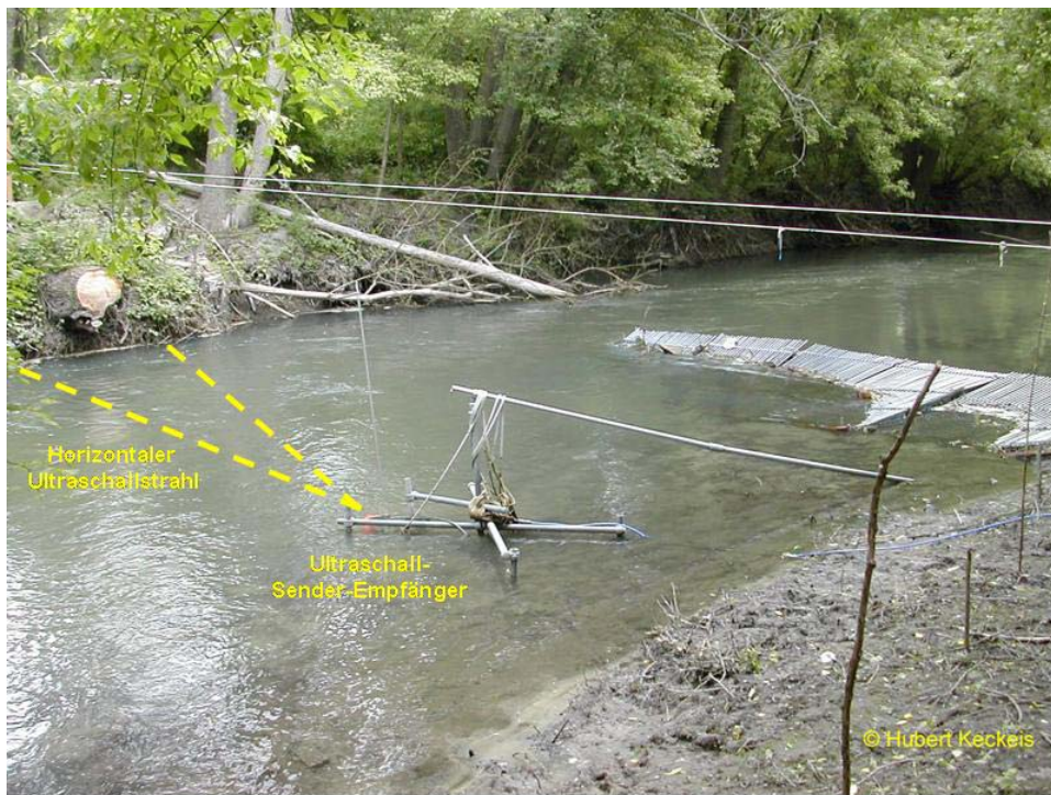
Pic. 1: The sampling site, 4km upstream the mouth of River Fischa. The river bed has a triangular cross-section with a gradually sloping right shore, the left shore increases steeply.
