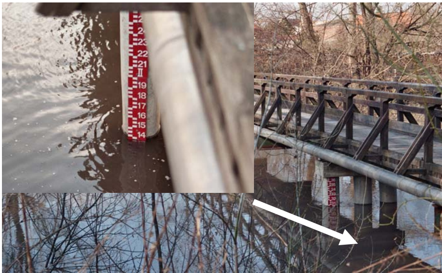
Pic. 5: Water-gauge at the wooden bridge in Fischamend, between hydroacoustic and trap net sampling site after flood.
