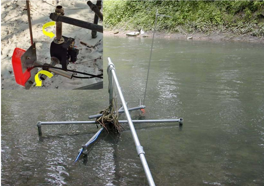
Pic. 2: Tetrapod-scaffolding with mounted elliptic splitbeam-transducer. The small picture shows the splitbeam-transducer which is connected with the rotator, the yellow arrows display possible movements of the rotator which sets the transducer.
