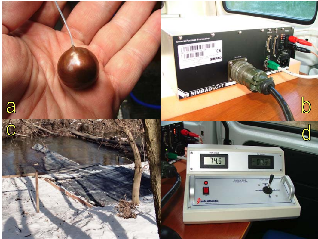
Pic. 4: a) The calibration-sphere made of tungsten is used for in situ calibration of the supersonic beam, b) shows the GPT-Unit which digitalizes the analogue data from the transducer, c) downstream placed panel-fence guides upstream moving fish out of the transducers nearfield, d) shows the Rotator-Joystick to set the optimal Pan- and Tilt-Angle.
