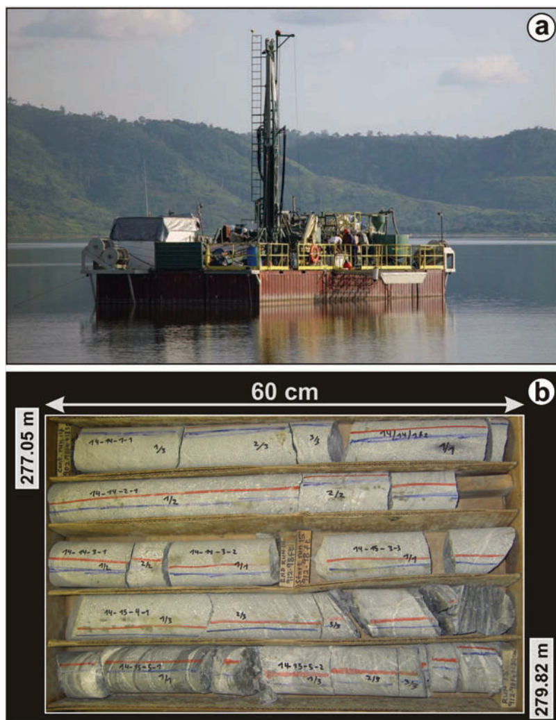
Figure 3-4. Photographs taken during the 2004 ICDP drilling project. a) General view of the GLAD800 drilling barge on Lake Bosumtwi (photo courtesy C. Koeberl). b) Example of core box (number 14; drill core LB-08A) showing metasediments, mainly meta-graywacke and some phyllite and slate (darker units) at the bottom of the image. Starting and ending depths of the cored section are also indicated, at the upper left and lower right, respectively.
