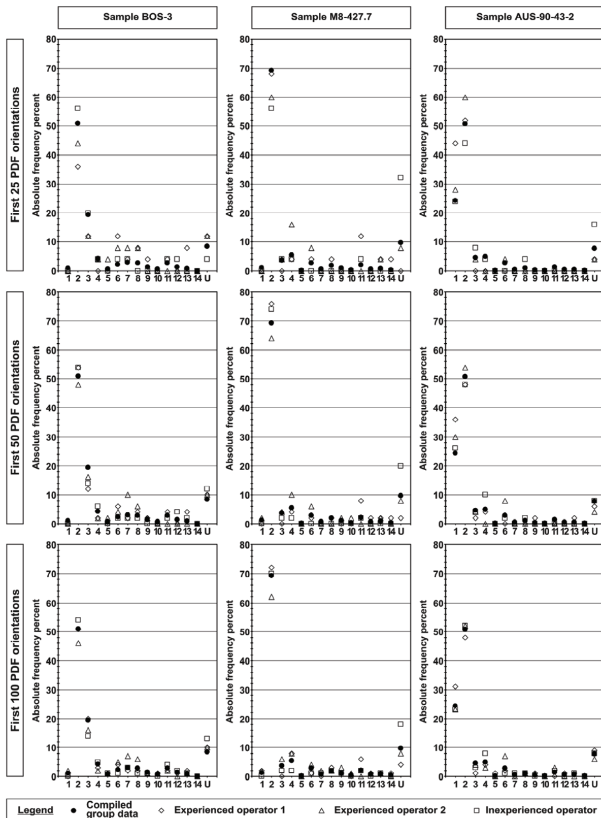
Figure 8. Absolute frequency distribution of indexed PDFs in quartz grains from BOS-3, M8-427.7, and AUS-90-43-2, as determined by each single operator and compared to the compiled group data (i.e., average of all PDF sets measured by the three operators), which is plotted for reference. Values reported on the x-axis correspond to the different PDF orientations shown in Fig. 1; the relative proportion of unindexed PDF sets (U) is also reported. Only the first 25 measured PDF orientations are reported in the first row, with the first 50 and first 100 measured PDF sets plotted in the second and third rows, respectively.
