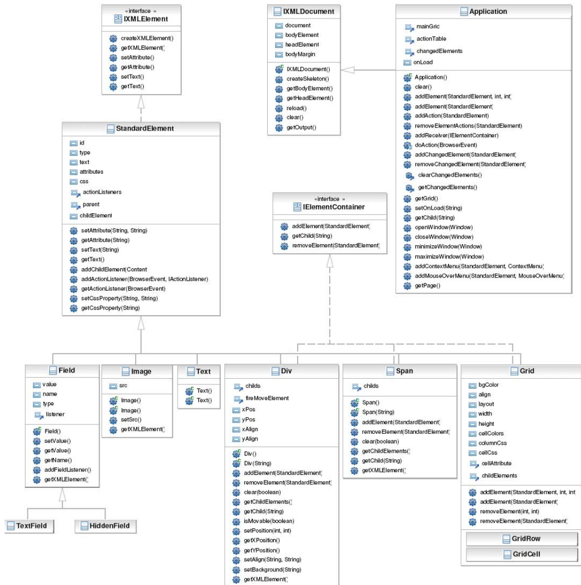
Figure 6.5: Basic API Structure
