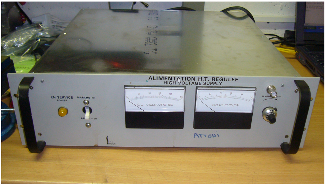
Figure 2.15: High Voltage Supply for the SPG
