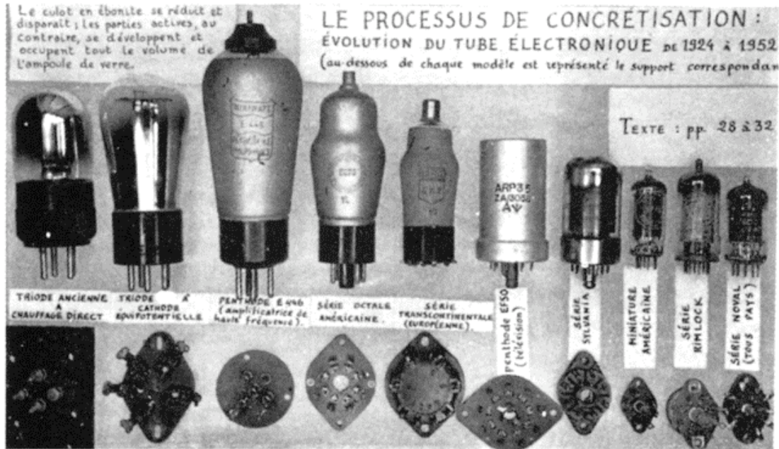
Fig. 1 Photograph by Simondon showing the evolution of the electronic tube from 1924 to 1952 as a concretization process. His commentary (top left) reads: “The ebonite socket reduces itself and disappears. In contrast, the active parts evolve and occupy the entire volume of the glass ampoule” (Simondon 1989).
