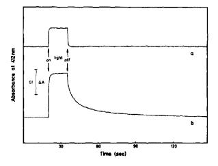
Fig.4. Kinetics of the 412 nm chromophore formation. Purple membrane (a) and purple membrane crosslinked with DTBP (b) of equal  $A_{570}$  were irradiated with light of  $\lambda > 515$  nm and the  $\Delta A_{412}$  monitored.
