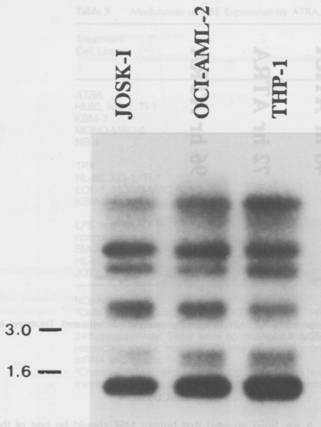
Figure 8 Restriction pattern of the MSE gene in high molecular weight DNA isolated from several MSE mRNA-positive and -negative leukemia cell lines. After endonuclease digestion with HindIII the DNA fragments were separated by pulsed field gel electrophoresis, Southern blotted, and hybridized to the HMSE-1 probe. The sizes of the bands are specified in the figure. The bands from all cell lines have approximately the same intensity; there were no gross alterations of the restriction patterns
