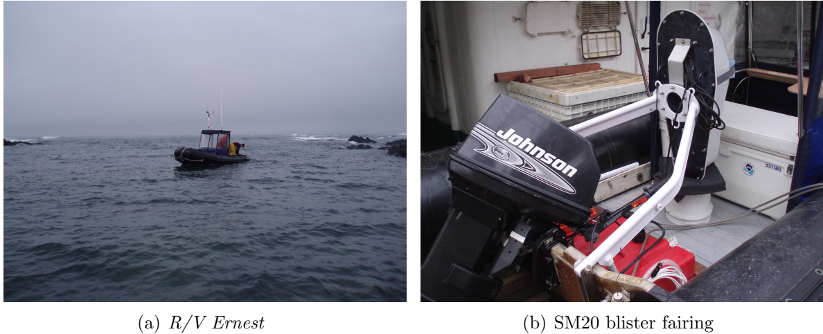
Figure 5.5: Near shore survey equipment. Figure 5.5(a) shows R/V Ernest entering the protected anchorage at Cape Shirreff, Livingston Island. Note the protective dodge to shelter personnel and equipment from the elements. Figure 5.5(b) shows the SM20 multi-beam echosounder, mounted inside a white blister fairing. The blister fairing was attached to a rotating frame that is mounted to the transom of R/V Roald .
