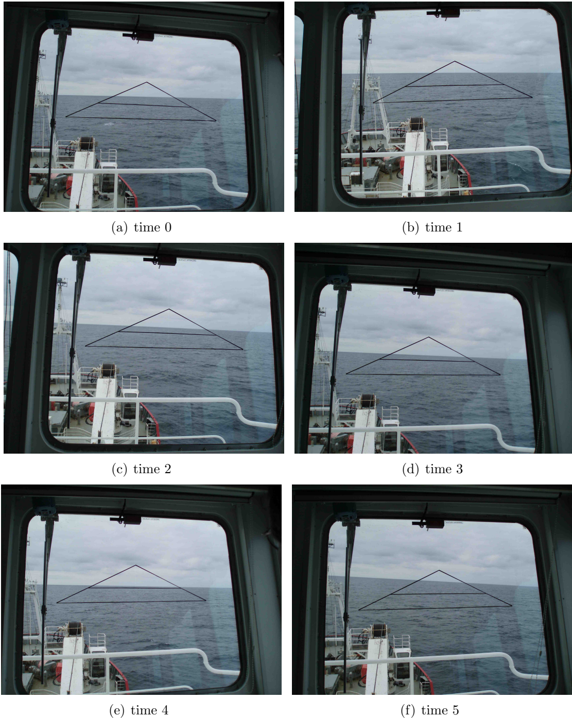
Figure 4.8: The location of 100 x 100 m box (parallelogram above base of triangle) for observing predator observations from the RRS James Clark Ross was highly susceptible to ship motion, and is potentially a large source of error when spatially aligning predator and acoustic observations. Photographs are between 1 and 2 s apart.
