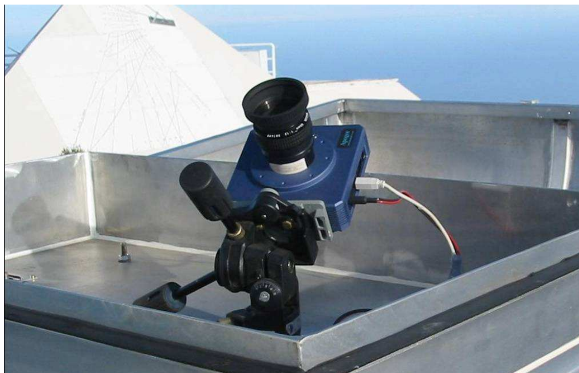
Figure 2.3: The PASS0 camera in its enclosure at the Teide observatory in Tenerife.
