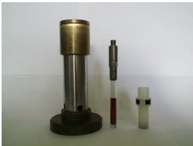
Fig 6.1. Brass and aluminium NMR tube protective case, 10 mm high pressure NMR cell and spinner.
