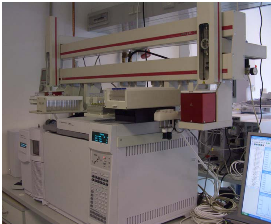
Figure 12: GC-MS with MPS-2 Prepstation
