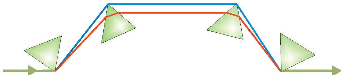
Fig. 1.3. A two prism pair arrangement which can be used to generate negative GVD
