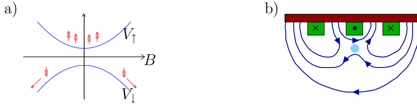
Figure 2.2: a) The potential for neutral atoms arising due to the Zeeman effect. Only states with a negative magnetic moment can be trapped, which are called low field seekers , because local magnetic maxima cannot be realized. b) A three wire configuration with a local minimum in the magnetic field is shown, which forms a one-dimensional waveguide.
