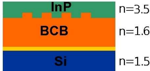
Figure 4.8: InP(m) layer structure. The thickness of the top InP layer is fixed at 300nm, but the other layer thicknesses are variable. The yellow layer is a high reflectivity film which is used in some device designs. The substrate is typically silicon, but GaAs is used where cleaving of the bonded structure is required.
