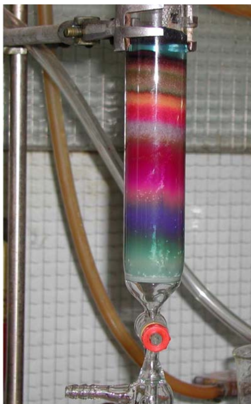
Figure 2.23. Photography of a chromatographic column separating the raw product in the synthesis of an unsymmetrical dye.
