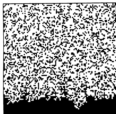
Figure 10b. Theoretical representation of a polymer matrix: changes during erosion (dark pixels = non-degraded areas, white pixels = degraded areas). (Reproduced with permission from ref. 33. Copyright 1993 ACS.)
