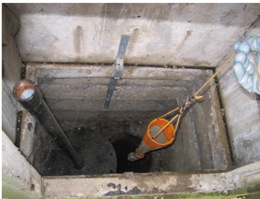
Lowering an ecology sampling net down a borehole.
