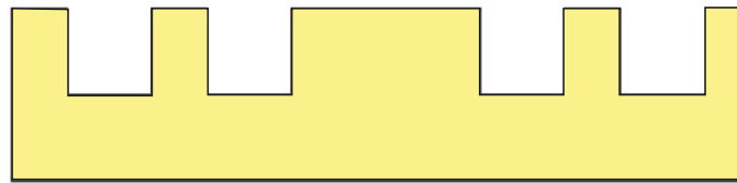
FIGURE 2. Post lithography and etch contact alignment mark
