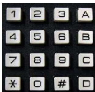
Figure 50: Interface 3. Actual use: A general purpose number entry interface for embedded systems
