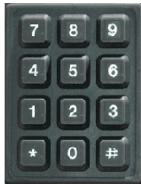
Figure 30: Interface 10. Actual use: A general purpose number entry interface for embedded systems
