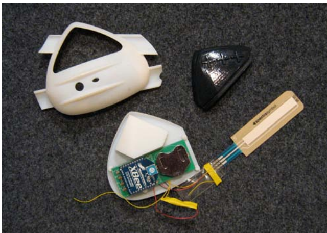
Figure 7. The shell and the electronic components that it hosts.
