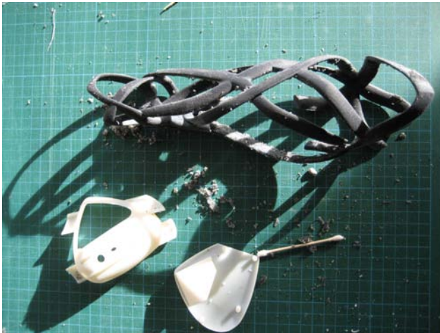
Figure 6. The three parts of the prototype, right after printing: the rubber armband before finishing and the two shells, which will contain the electronic components.
