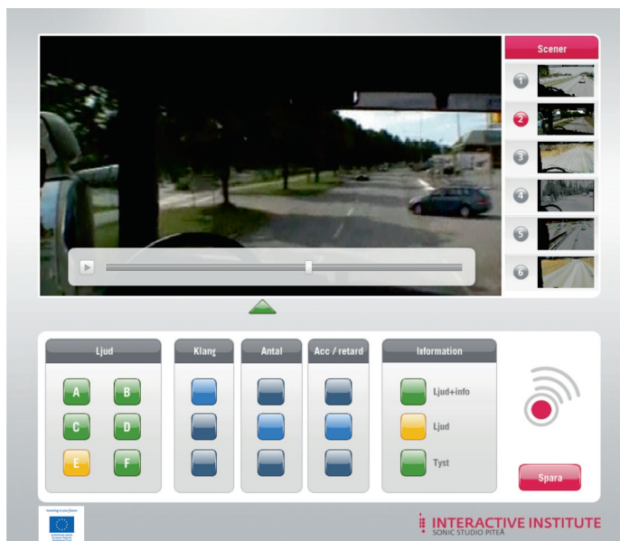
Figure 2 Participatory Audio Research Tool (PART). The user situations are represented by images or videos. By using the radio buttons in the lower part of the screen, users can adapt the sound to the situation.
