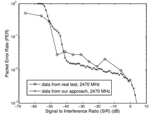
Fig. 8. PER under microwave oven Interference with frequency 2470 MHz
