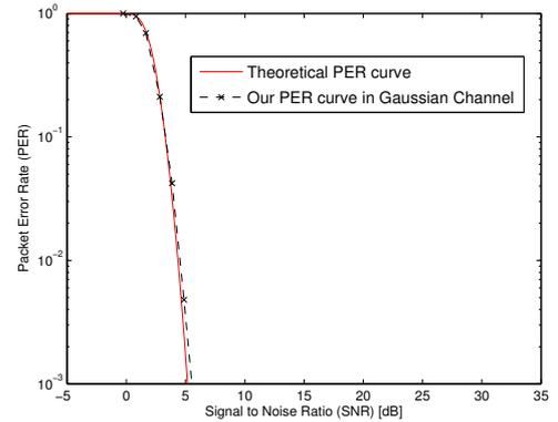
Fig. 4. Packet error rate (PER) in a Gaussian channel. Theoretical and measured results match very well. changes from our test in no fading channel, with the theoretical PER curve as a reference.
