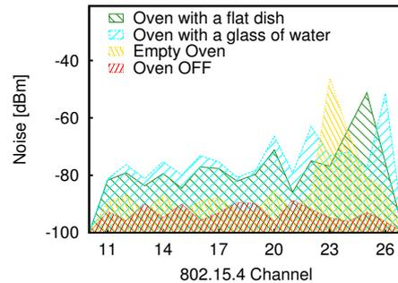
Fig. 6. Spectral characteristics of microwave interference
