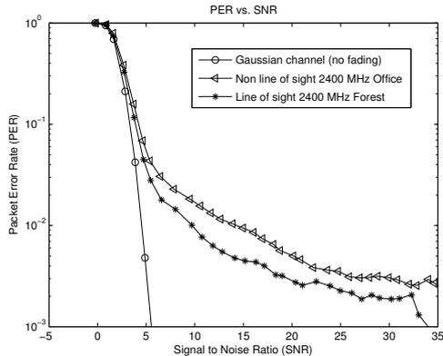
Fig. 5. Packet error rate (PER) for a range of signal-to-noise ratios (SNR). The channel was block fading, that is to say roughly constant during a packet but changing on an inter-packet time scale.
