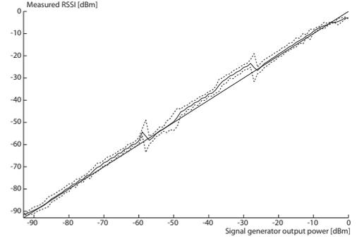
Fig. 3. RSSI from the CC2420 as a function of the VSG signal output power. The mean  $\pm 3$  standard deviations are given together with the ideal straight-line response. The curves are based on 10000 RSSI readings per power setting.
