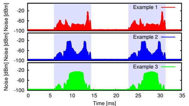
Fig. 7. Temporal characteristics of microwave interference
