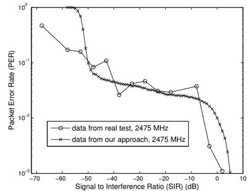
Fig. 9. PER under microwave oven Interference with frequency 2475 MHz
