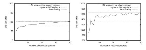
Figure 1: LQI variance for a channel with high PRR (good) and a channel with a lower PRR (bad). The left figure shows the good channel (PRR of 99.9%) with LQI variance of about 100, while the LQI variance of the bad channel (PRR of 87%) in the right figure is around 16 times higher.
