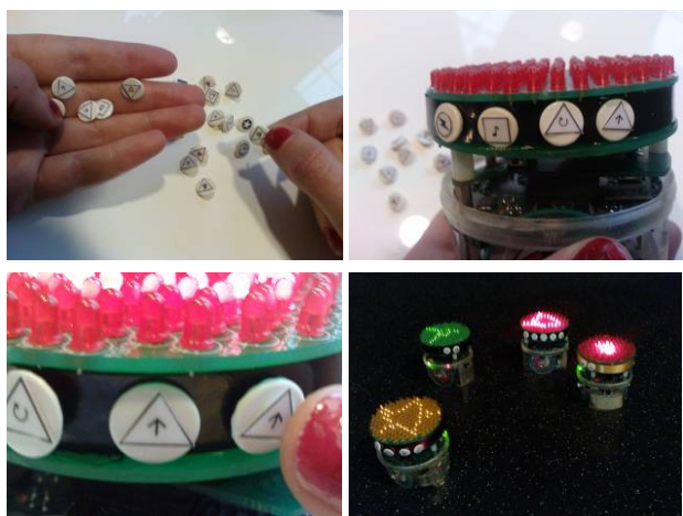
Figure 2. The GlowBots scenario. Selecting from a collection of physical behaviour “amulettes”, attaching them to a GlowBot, and finally the GlowBots move, glow, and interact according to items on their bracelets.
