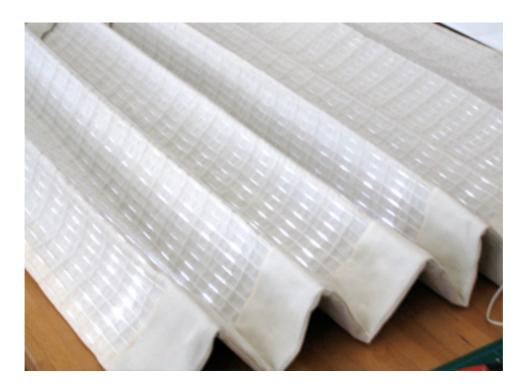
Several version of the Energy Curtain have been built, including versions fashioned as a horizontally-folding Roman blind or as separate vertical Lamellae panels. The technical principle of all the prototypes is based on solar panels, small batteries, LEDs and optical fibres. These
