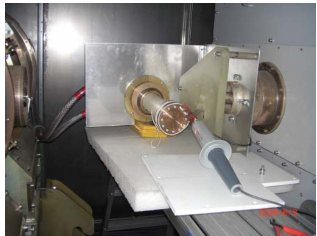
Figure 4: Dummy load in place of the cavity, which is seen at the left-hand side.
