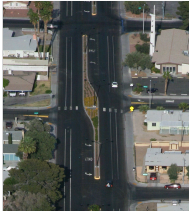
Aerial view of an access management configuration
