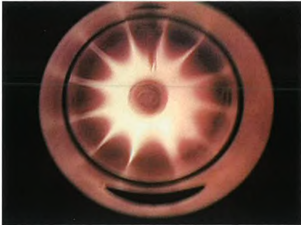
Fig. 4.12 Photograph of a D 2 ICP with External Magnetic Field Applied Generating a Multicusp Geometry.
