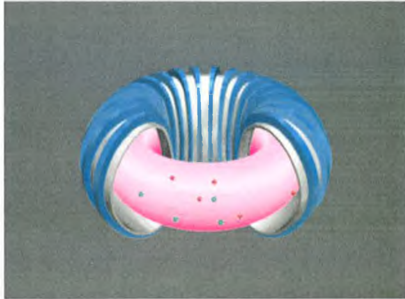
Fig. 1.1 Representation of TOKAMAK for Use in Neutral Beam Injection (NBI).
