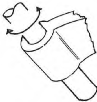
Figure 2.2(a) Typical revolute Joint
