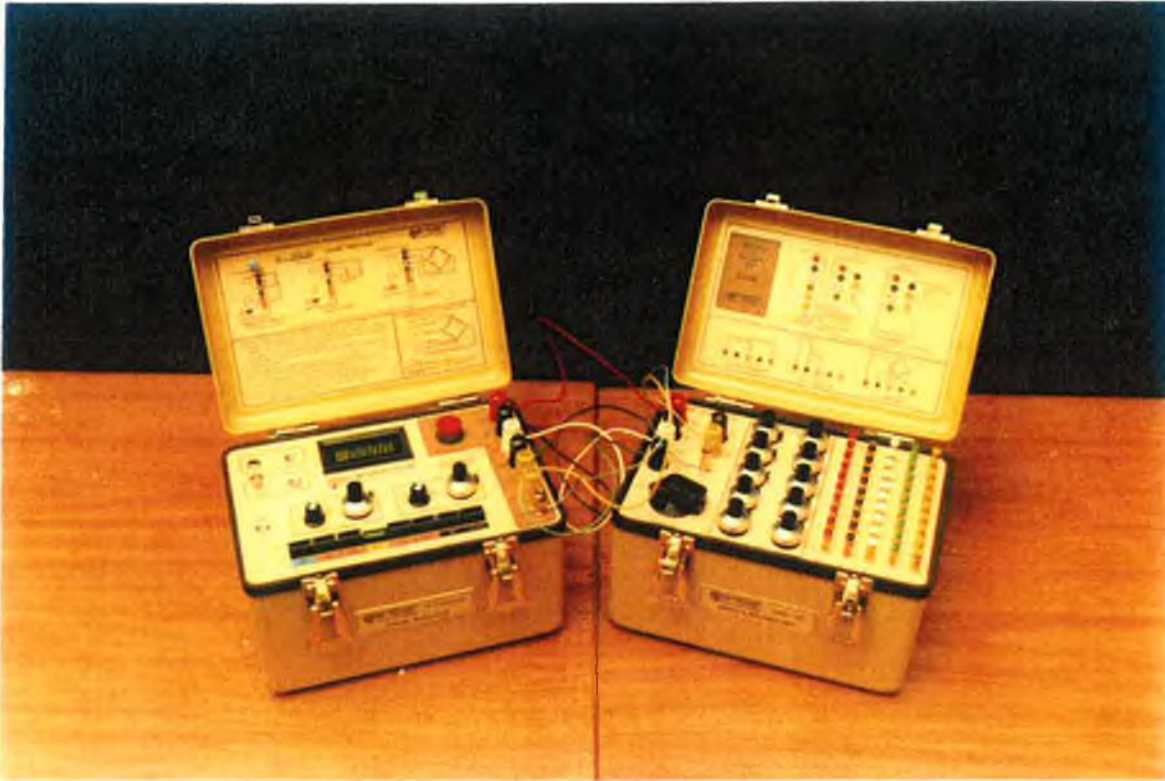
PLATE 3.7 THE DIGITAL INDICATOR P-3500 & THE SWITCH BALANCE SB-10.
