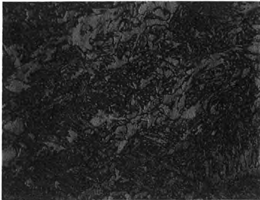
PLATE 4.6 THE MICROSTRUCTURE OF THE WELDING ZONE AFTER PWHT (TIME DURATION OF 10 h) FOR AISI-1020 WELDED COMPONENT, X500.
