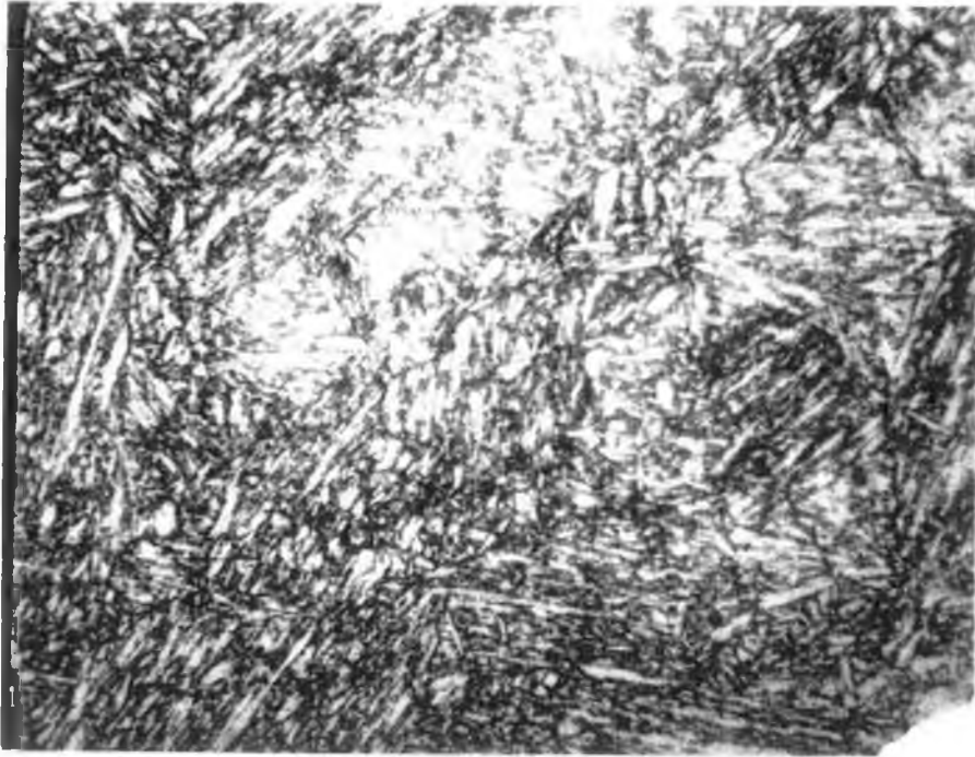
PLATE 4.7 THE MICROSTRUCTURE OF THE WELDING ZONE BEFORE PWHT FOR AISI-410 WELDED COMPONENT, X500.
