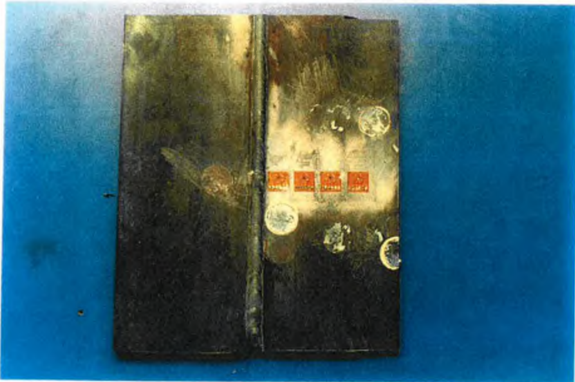
PLATE 4.12 THE RESIDUAL STRESSES MEASUREMENT POINTS ON THE WELDED COMPONENT.
