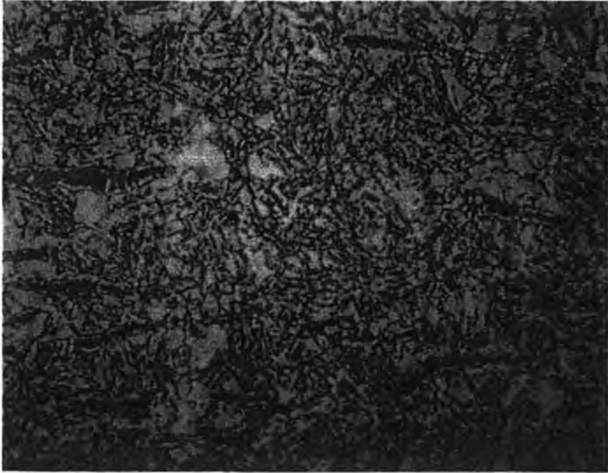
PLATE 4.9 THE MICROSTRUCTURE OF THE WELDING ZONE AFTER PWHT, SOAKING TEMP. OF 650°C FOR AISI-410 WELDED COMPONENT, X500.
