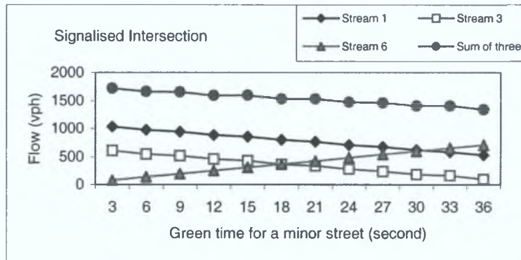
Figure 4.19. Flow of different streams varies with the duration of green light of minor-street
