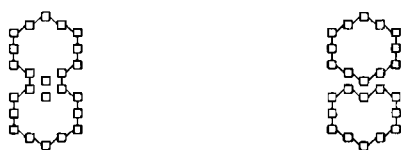
Figure 7 The division of an hourglass-shaped membrane into two membranes. The channel is now made up by two different parts of the same membrane. Again, the free links have to be located in this channel.
