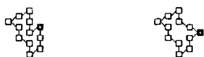
Figure 8 The link which initiates the chain motion is marked with an absorbed substrate. Note that at its position there are two adjacent acute angles in the membrane. The link moves towards southeast, dragging the link previously southwest of it behind. This action eliminates one acute angle from the membrane which wouldn't have been possible with membrane flexibility alone.
