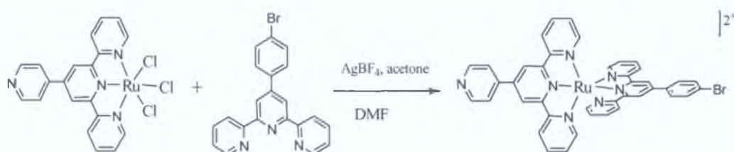
Figure 3.16: Synthesis of [\text{Ru}(\text{py-tpy})(\text{tpy-ph-Br})][\text{PF}_6]_2 complex
