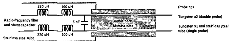
Figure 3 7 General probe design with radio-frequency inductors and coupling capacitor
