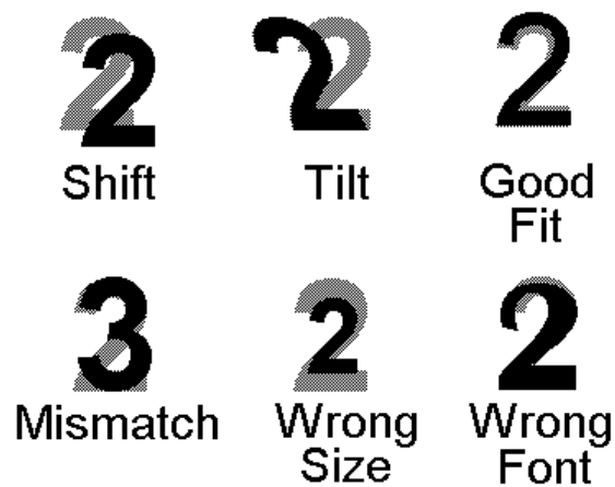
Figure 2.7 Recognising a numeral '2' using an N-tuple.
