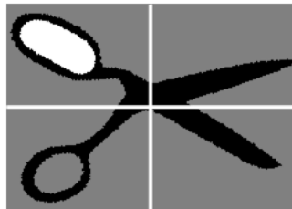
Figure 7.4.11 Chirality test based on the fourth program for chirality . The input image has been normalised, using [ npo,chf ], so the centroid of the blob is at the centre of the image and its principal axis is horizontal. Since the centroid of the largest lake is above the centre of the image, the chirality is taken to be " right ". Notice that the chirality calculated in this way is different from that derived by the third method.
