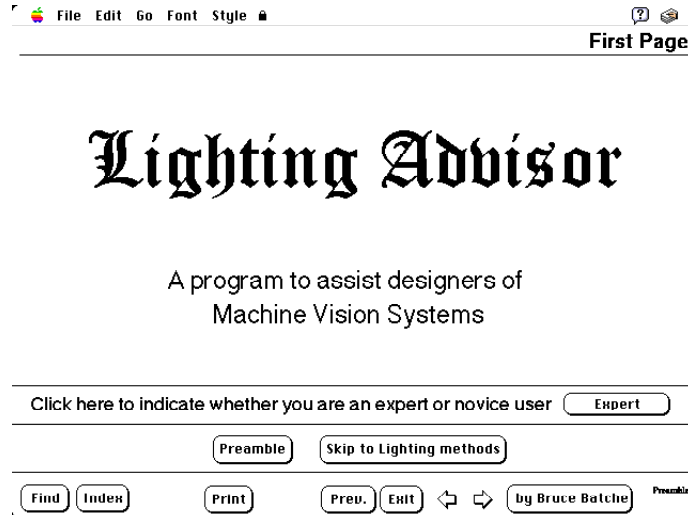
Figure 4.15 The first card in the “Lighting Advisor” stack. Notice the presence of several buttons to initiate navigation through this stacks. The functions of these buttons are explained in the text. The user can indicate his level of his expertise, by clicking on the button on the lower right. (The button label toggles between “Expert” and “Novice”.)
