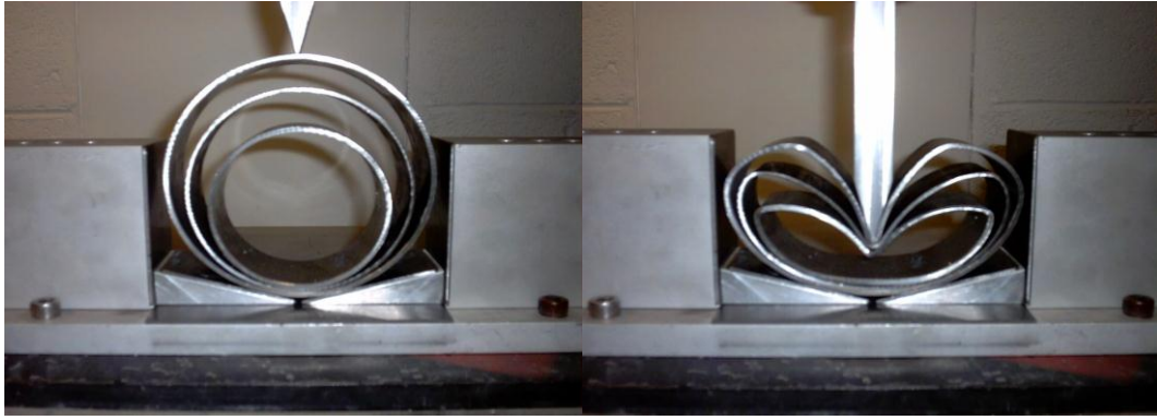
Fig. 12b. Initial and final stages of compression for a 3 tube system with in 15 degrees inclined constraints.
