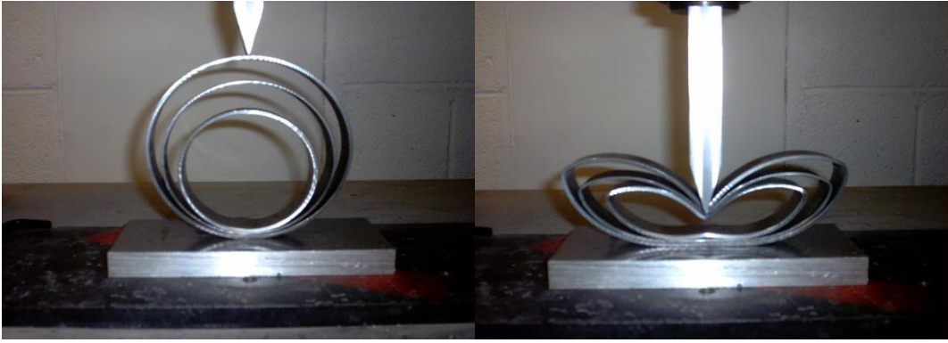
Fig. 11a. Initial and final stages of compression for a 3 tube system with no constraints.
