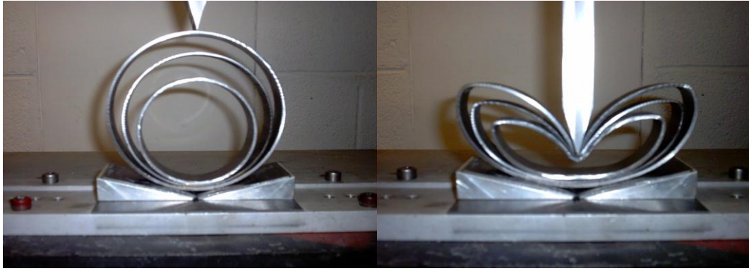
Fig. 11b. Initial and Final stages of compression for a 3 tube system with 15 degree inclined constraints.
