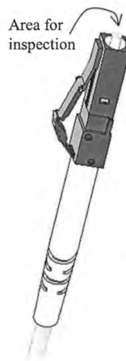
Figure 2-1 – LC fibre connector
