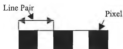
Figure 2-20 – A pair of imaging pixels are required to define a line pair
